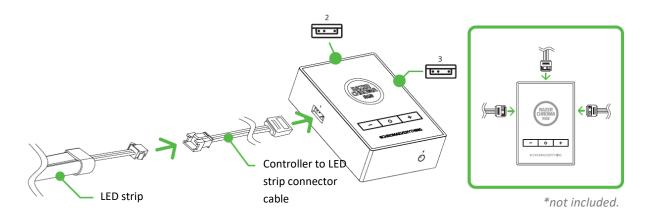
Before plugging a controller to LED strip connector cable to the ARGB controller, make sure that the ARGB controller is powered off and the chosen port is properly aligned to the cable's connector.
