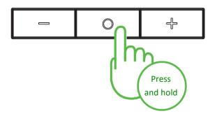
2. Press and hold the power and brightness control buttons simultaneously for 3 seconds to activate pairing mode. The first LED of each connected strip will blink in blue to show that the device is in pairing mode.
