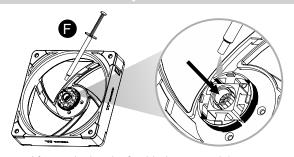
After replacing the fan blades several times, readd the oil into the bearing (about 0.1ml)
