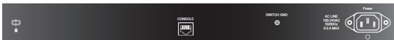
Figure 1.11 — DGS-1210-52/ME rear panel
