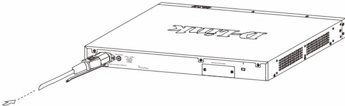
Figure 9 — Connect the power cord to the switch
