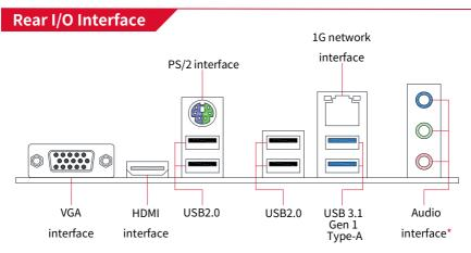
(\*Note: The blue in the audio interface is the audio input, the green is the audio output, and the pink is the microphone interface)
