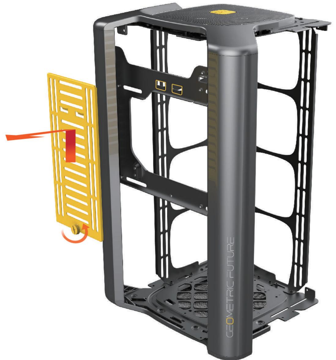
4 Remove the water-cooling brackets
