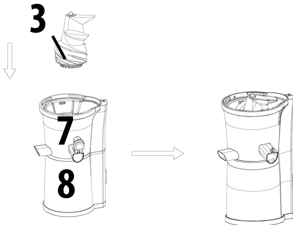
Then place the feed auger (3) in the already installed juice strainer / sorbet insert, press it down and turn it until it engages.
