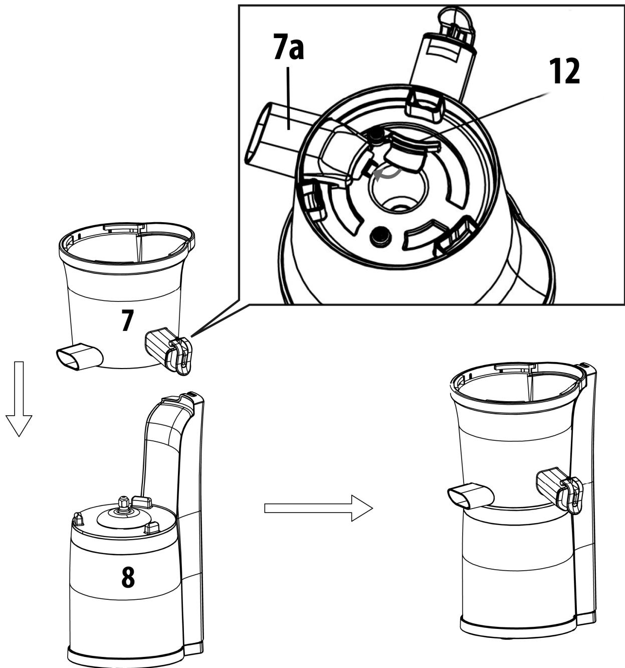
Ensure that the silicone plug (12) is placed in the residue outlet (7a); see the underside of the strainer compartment with outlets (7). Place the strainer compartment with outlets (7) on the motor unit (8).
