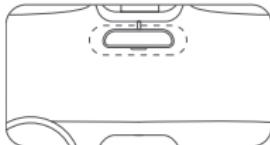
Avoid the edge of the windshield and select the flat and smooth area for the installation.
