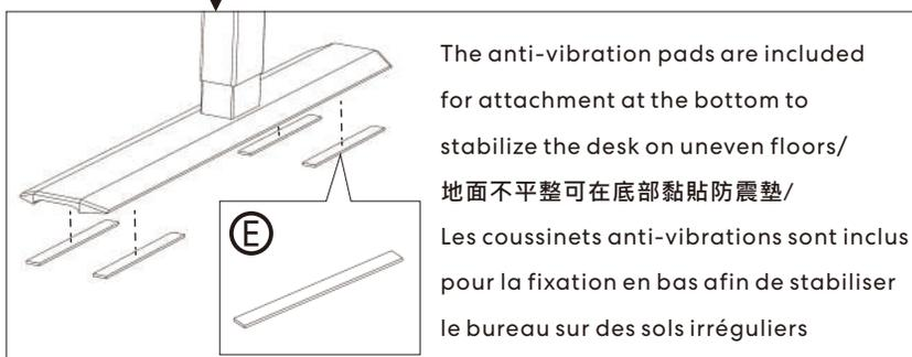
The anti-vibration pads are included for attachment at the bottom to stabilize the desk on uneven floors/
