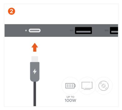
Connect USB-C charging cable to the adapter's USB-C PD charging port.
