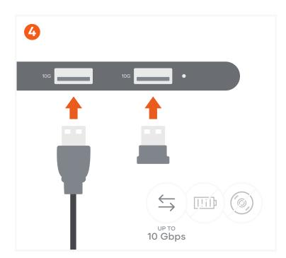
Connect up to two USB-A peripherals or devices for data transfer - up to 10 Gbps.
