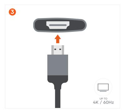
Connect HDMI cable from the adapter to a 4K HDMIequipped display. Up to 4K at 60Hz.
